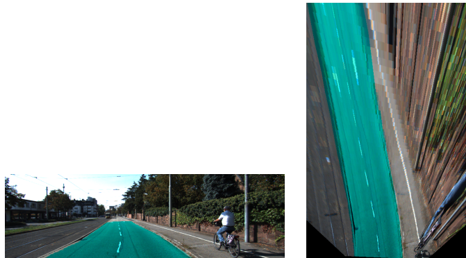
Figure 5: Drivable area on camera view and top view projected from the neural network output
