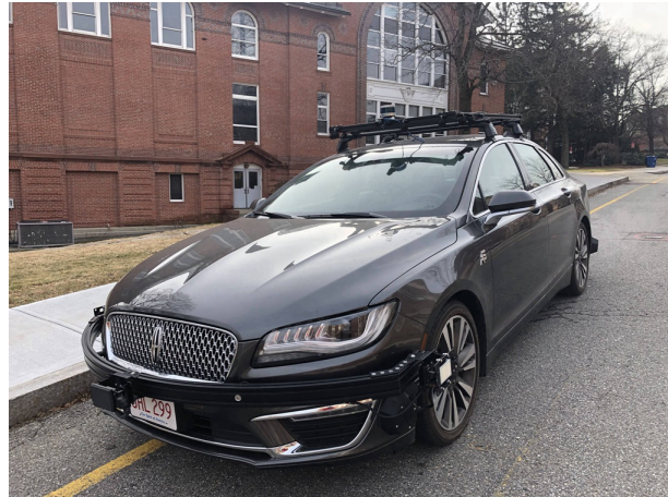
Fig. 1: A Lincoln MKZ equipped with 1 LiDAR, 1 front camera and 10 side cameras
